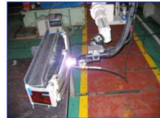
Welding test for Vacuum Vessel
